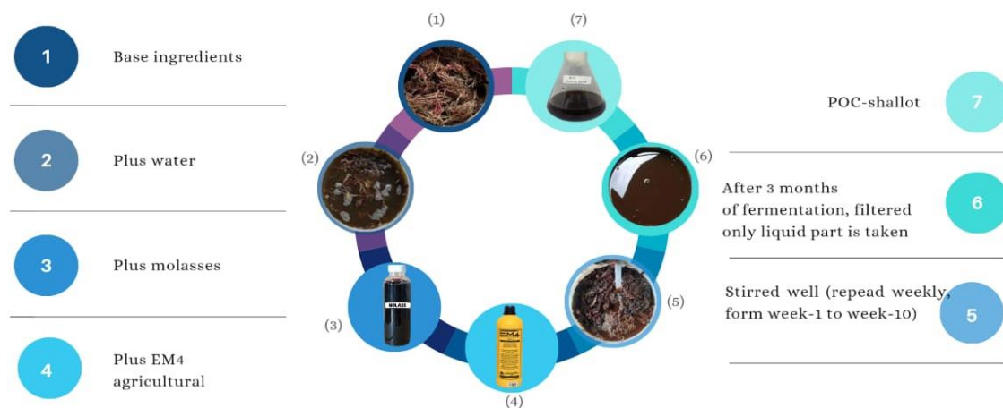
Figure 1. Production stages of Shallot Liquid Organic Fertilizer (LOF-Shallot)
