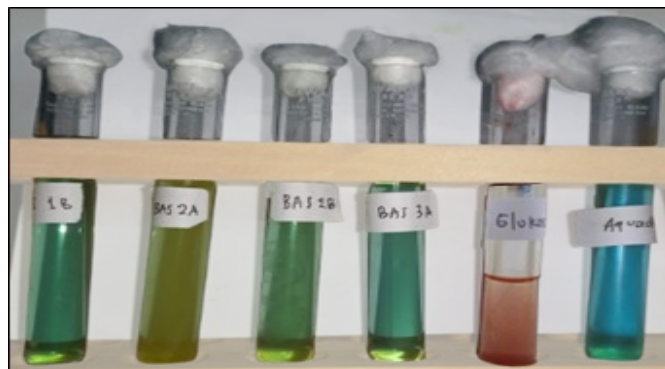
Figure 4. Saccharification test results using Benedict's reagent
