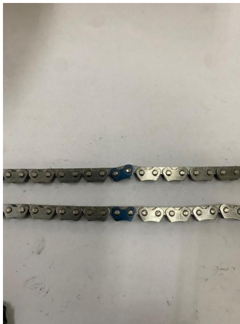
Figure 4. Comparison Between a Stiff Chain Condition and a Normal (OK) Chain Condition
