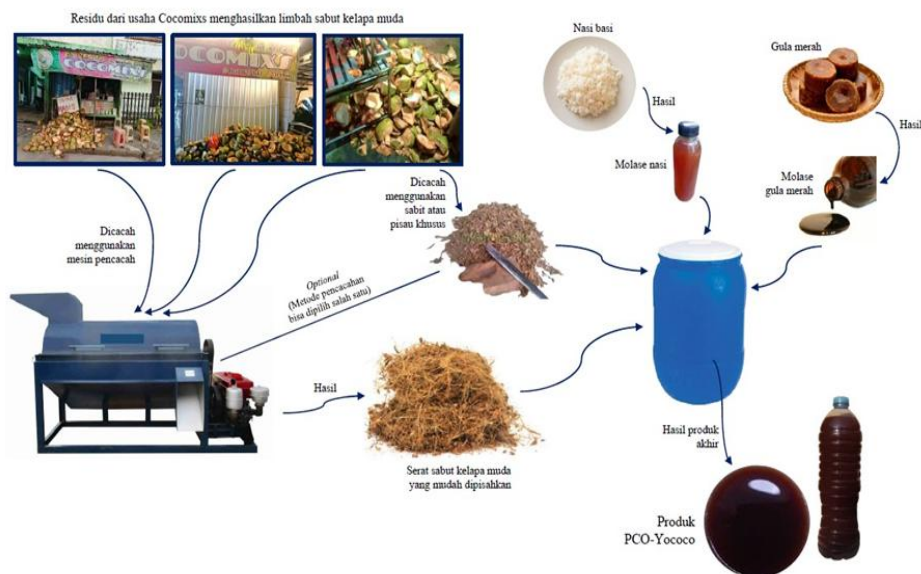
Figure 1. Schematic Illustration of the Technology and Innovation Applied in the Empowerment of PKK Cadres Through Training on Processing Cocomixs Waste Into PCO-Yococo for the Sustainability of Kebun Rahayu in Teguhan Village
